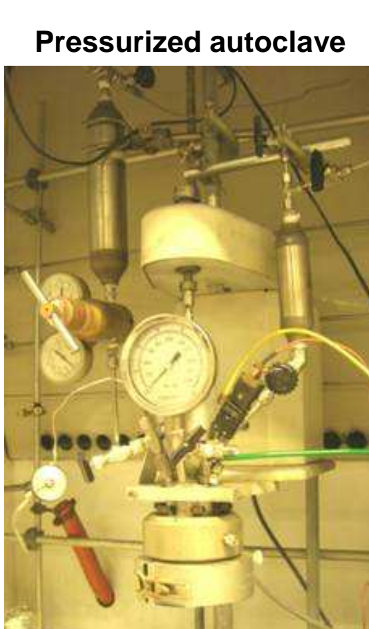
50 mL n-heptane, 20-40 mg of catalyst NiX/SiO 2 , Styrene/Ni 2 =5000, 700 rpm, at 5°C/15bar then 150°C/60bar
