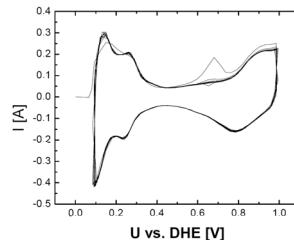
Right side: schematic illustration of half cell measurement carried out in a fuel cell (photographs). Left side: Cyclic voltammogram of Pt/C in water measured in half cell mode
