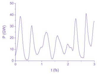
SASE1 power at saturation: typical feature size is 0.3 fs (100 nm)
