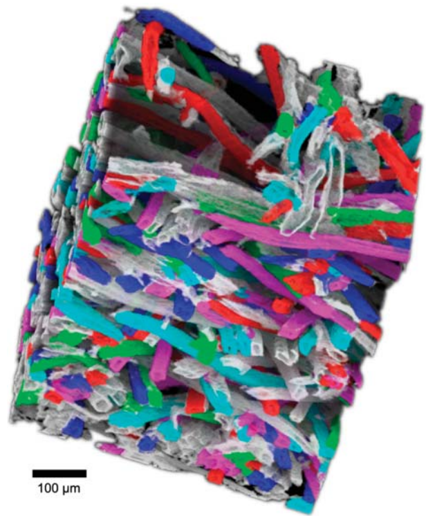
Figure 4 Example of a rendered MDF 256^3 voxel sub-volume with a target density of 300 \text{ kg m}^{-3} with individually marked fibers.
