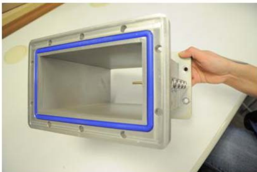
Fig. 7: Waveguide with damping antennas at the small side of the waveguide
