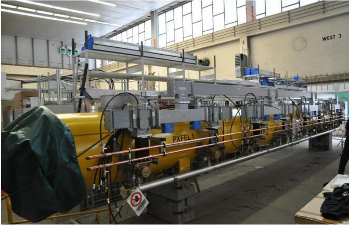
Fig. 5: Accelerator module and RF waveguide distribution
