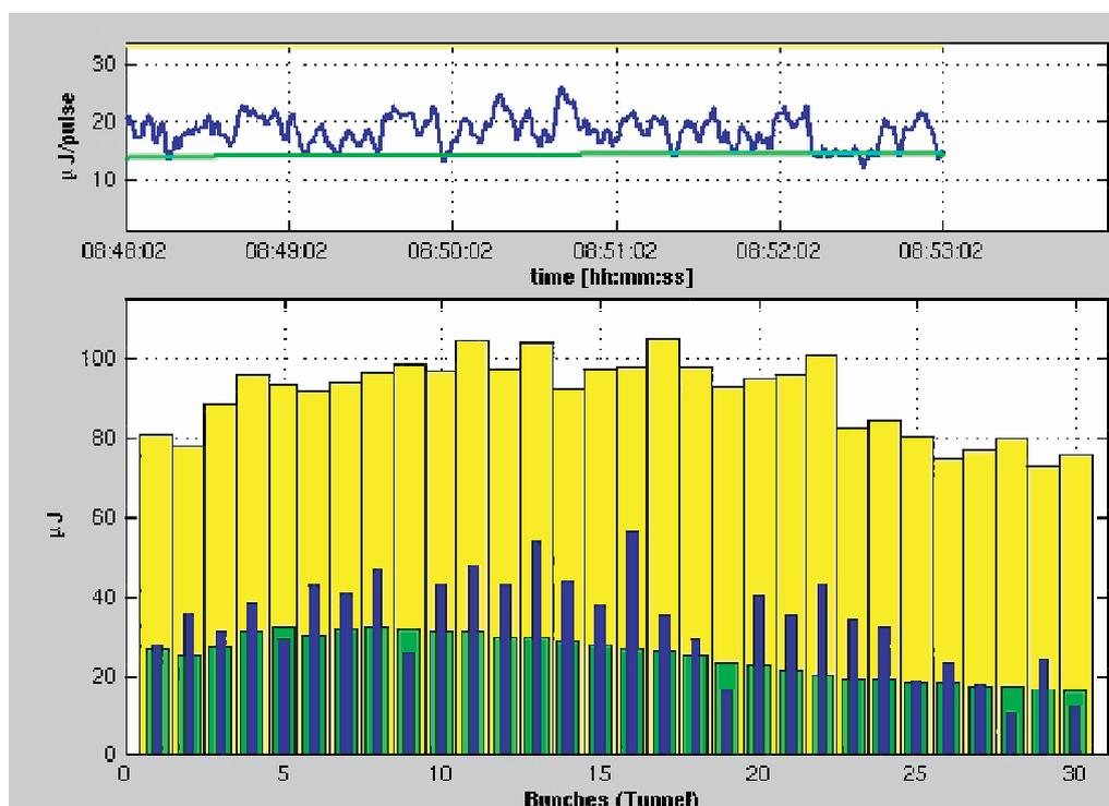
**Figure 5.** Display of the GMD in the control system. The blue line in the upper part represents the pulse energy (in  $\mu\text{J}$ ) averaged over 25 s as a function of time (green line = averaged over longer period). Lower part: the blue bars represent the pulse energy (in  $\mu\text{J}$ ) of each bunch of the actual bunch train (yellow bar = maximum value, and green bar = averaged for the respective bunch since start of averaging).
