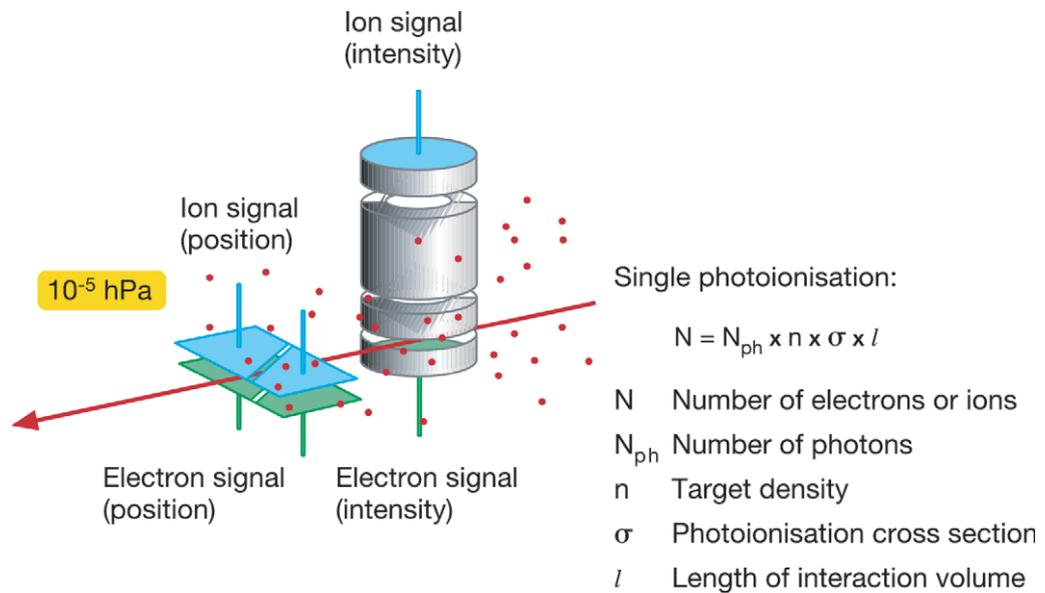
**Figure 4.** The GMDs provide non-invasive measurements of the shot-to-shot intensity. To the right: a Faraday cup counts the electrons and ions that are produced as the FEL pulse passes through the ionization chamber containing nitrogen or rare gases at very low pressure. To the left: the two split electrodes determine the horizontal position of the beam.
