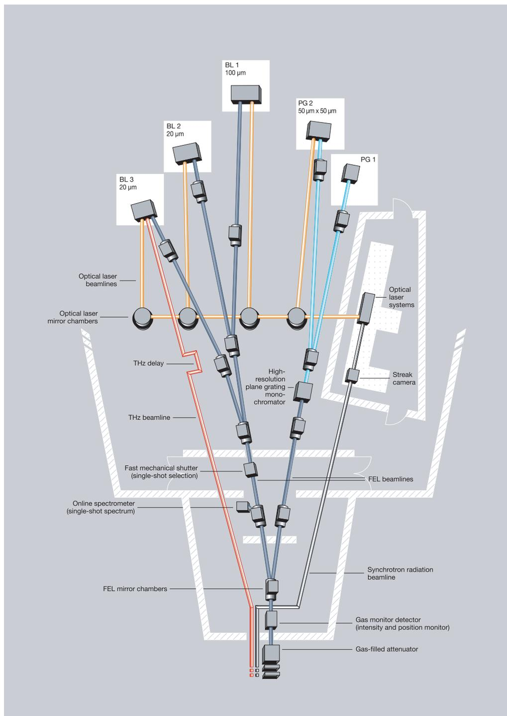
**Figure 2.** Schematic view of the experimental hall. Beamlines are highlighted by a colour code: ‘direct’ FEL beam in dark blue, monochromatized FEL beam in light blue, optical laser in orange and THz radiation in red. Different experimental stations are named ‘BL’ in case of direct FEL beam or ‘PG’ for the monochromatized FEL beam. Approximate focal sizes are given next to the station name.
