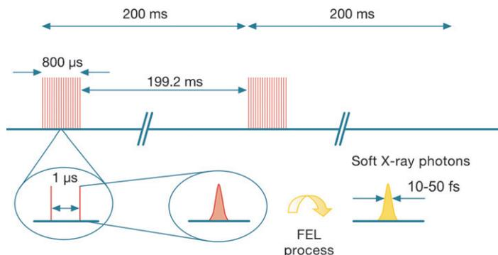
**Figure 1.** Electron bunch time pattern of FLASH with 5 Hz repetition rate and up to 800 bunches in a 800  $\mu\text{s}$ -long bunch train. The separation of electron bunches within a train can be set to 1, 2, 10 or 100  $\mu\text{s}$ . The pattern is directly transferred to the photon pulses as each electron bunch produces one photon pulse.
