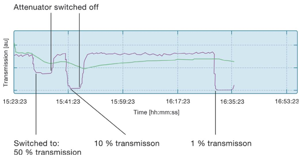
**Figure 6.** Attenuator performance during an experimental run. The blue curve shows the transmission signal in real time, whereas the green curve displays a time average with a time constant of 30 min.
