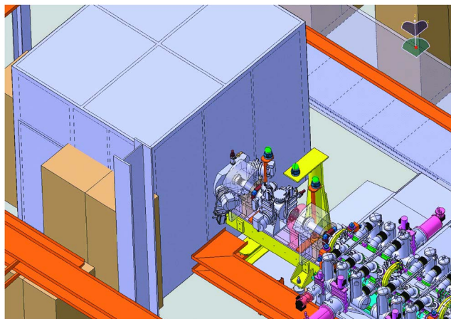
FIG. 1. (Color online) Linac4 front-end (status August 2007) with the IPHI RFQ (95 keV injection energy).
