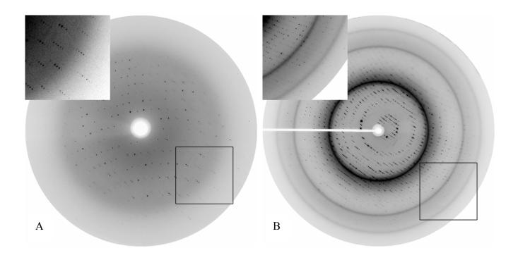
**Fig. 3.** X-ray diffraction patterns recorded for two different crystals of NodS. A: NodS without ligand (0.75° oscillation), B: NodS in complex with SAH (0.5° oscillation). The edge of the detector (framed, inset) corresponds to a resolution of 2.3 (A) and 1.71 Å (B).
