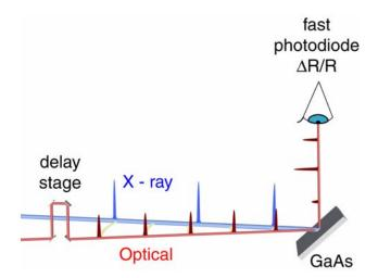
**Fig. 1**: Transient X-ray induced optical reflectivity (∆R/R) measurement - schematic overview:
