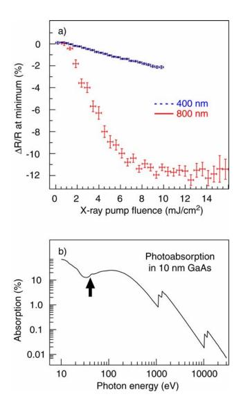
**Fig. 3:** Transient X-ray induced optical reflectivity ( $\Delta R/R$ ) – energy dependence: a) Dependence of the initial drop of  $\Delta R/R$  for 800 nm and 400 nm probe light on the fluence of the X-ray pulses. The error bar in X-ray pump fluence reflects the finite binning intervals used. The error bar of  $\Delta R/R$  is the standard deviation of events within the corresponding fluence binning interval.
