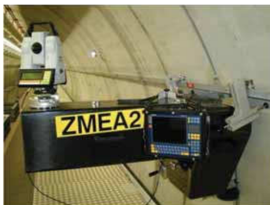
Figure 7.2.10 Carriages for laser tracker and tachymeter.
