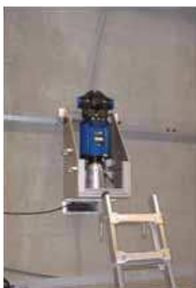
Figure 7.2.10 Carriages for laser tracker and tachymeter.
