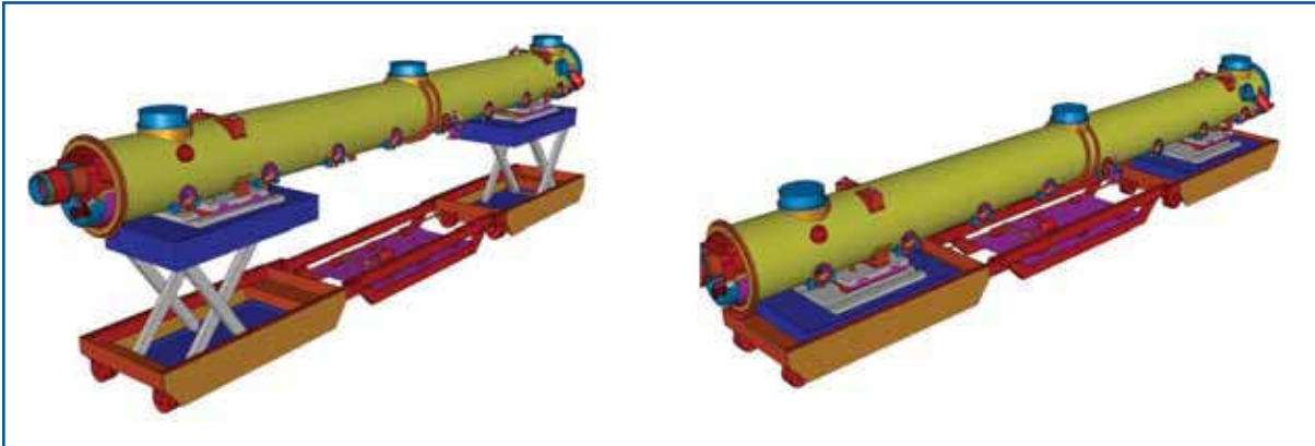
Figure 7.2.13 The conceptual design of the accelerator module transportation and installation vehicle.
