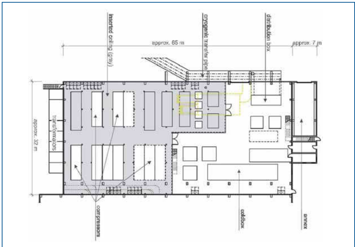
Figure 7.1.8 Ground plan of the XFEL cryogenics hall. The dimensions of the hall are about 72 m × 32 m with a height of about 14 m.
