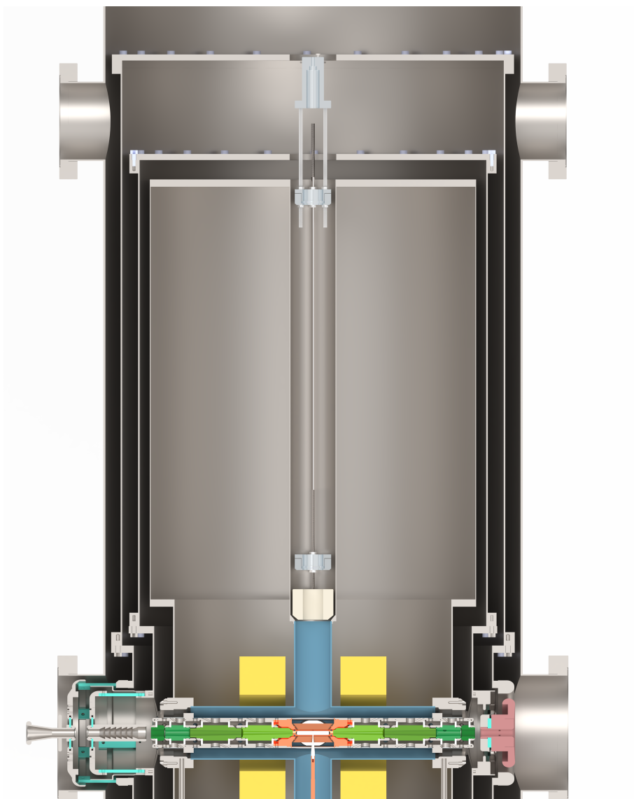
Figure B.1.2: Cross sectional view of the lens assembly in the HD-EBIT
