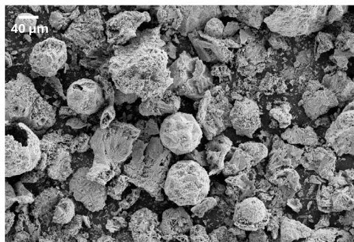
Fig. 3. SEM micrograph of initial \text{Fe}_2\text{O}_3 particles.
