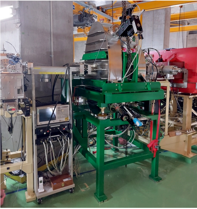
Figure 1: A photograph of a Schottky Cavity Doublet (SCD) installed at R3 storage ring. It is shown above on top of green mechanical support (elliptical cavity left). A separate publication will be dedicated to the technical details and features of the new detector. (Photo: S. Sanjari)
