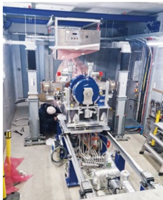
Figure 4: View into the opened radiation shielding of the Facility for L-band Conditioning (FALCO), with Gun 5.2 installed on the rail system and RF waveguides attached to the newly developed two-arm RF input coupler
