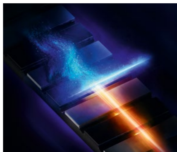
Electrons (blue cloud) are squeezed together in a chicane to emit very bright X-ray light (orange beam).
