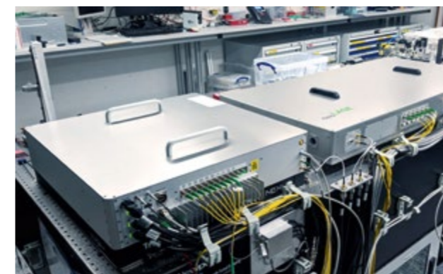
Figure 1: Fibre frontend and power amplifier of the NEPAL-X1 laser during installation
