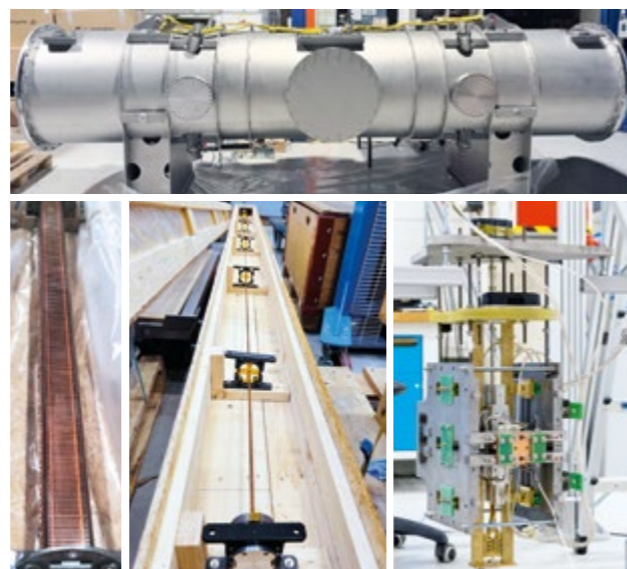
Figure 5: Top: Outer vessel of the S-PRESSO cryostat. Bottom left: 2 m long SCU coils. Bottom middle: 5 m long vacuum chamber prototype with a cross section of 10 x 5 mm 2 . Bottom right: Phase shifter.
