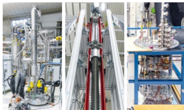
Figure 6: Main components of SUNDAE1. From left to right: Cryostat, linear motion stage, and lid.
