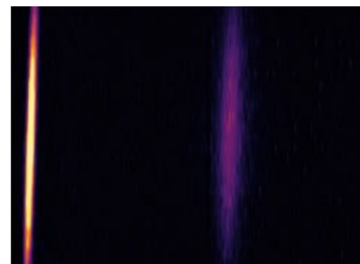
Elastically scattered X-rays (bright yellow light) and X-rays scattered from plasmons (faint violet light)
