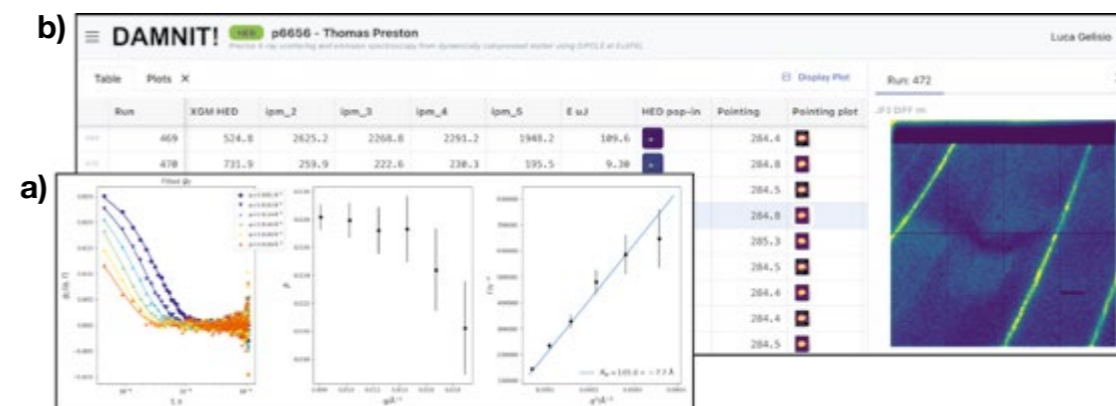
Figure 12: (a) Part of the results of the real-time X-ray photon correlation spectroscopy data analysis pipeline, available in DAMNIT. (b) Screenshot of DAMNIT used during an X-ray scattering experiment.
