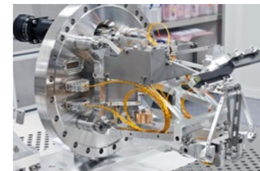
Figure 2: Mechanical design of the CBXFEL retro-reflector based on parallel kinematics and flexural elements. The unit positions two total-reflecting X-ray mirrors in the beam path. Altogether, four similar units are required for the cavity to position four mirrors and two diamond crystals.
