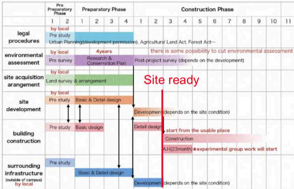
Figure 6: Gantt chart of the time line from green light to the begin of experiment construction [5].
