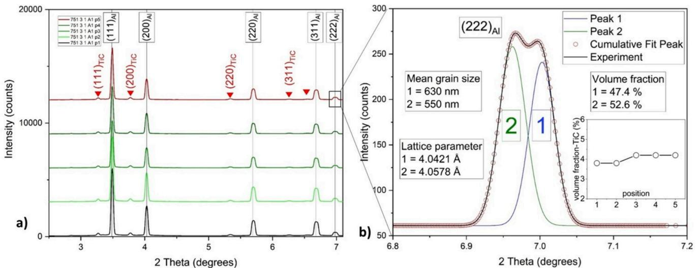
Fig. 5. Set of X-Ray synchrotron radiation diffraction patterns recorded at five different positions of sample (a), result of Rietveld analysis of (222) Al matrix peak (b) and plot showing volume fraction of TiC phase calculated for individual measuring positions (c).
