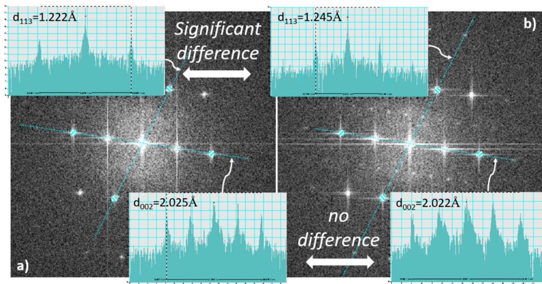
Fig. 10. FFT images for regions without (a) and with (b) the titanium in Al solid solution and results of measurement of interplanar spacings by the profile intensities along indicated lines.
