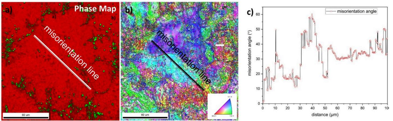
Fig. 3. (a) EBSD phase map; (b) inverse pole figure (IPF) orientation map with the corresponding misorientation profile; (c) distribution of the misorientation angle measured along the line indicated in (b).
