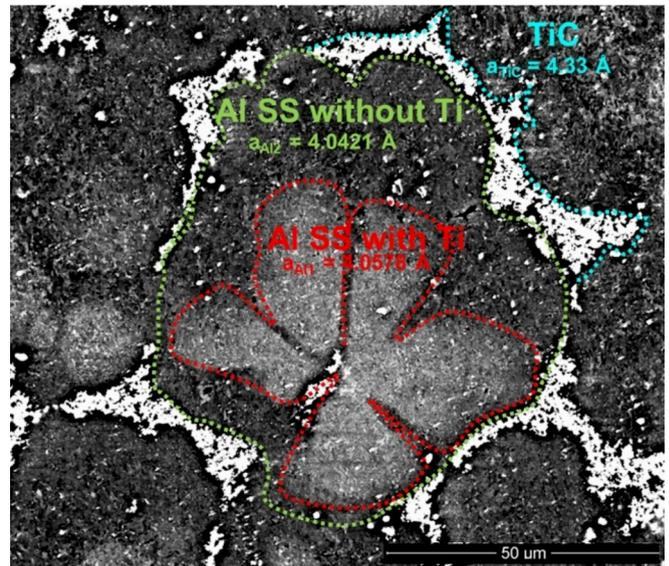
Fig. 11. SEM-BSE image of the flower-type microstructure with the marked ranges of occurrence of individual solid solutions and TiC particles.
