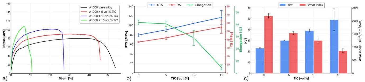
Fig. 12. Set of mechanical properties of aluminum Al1000 series alloy and composites containing 5–15 vol% TiC, tensile strain–stress curves a) results of microhardness measures, UTS-ultimate tensile strength, YS-yield stress and A-starin b), along with HV and wear index c).
