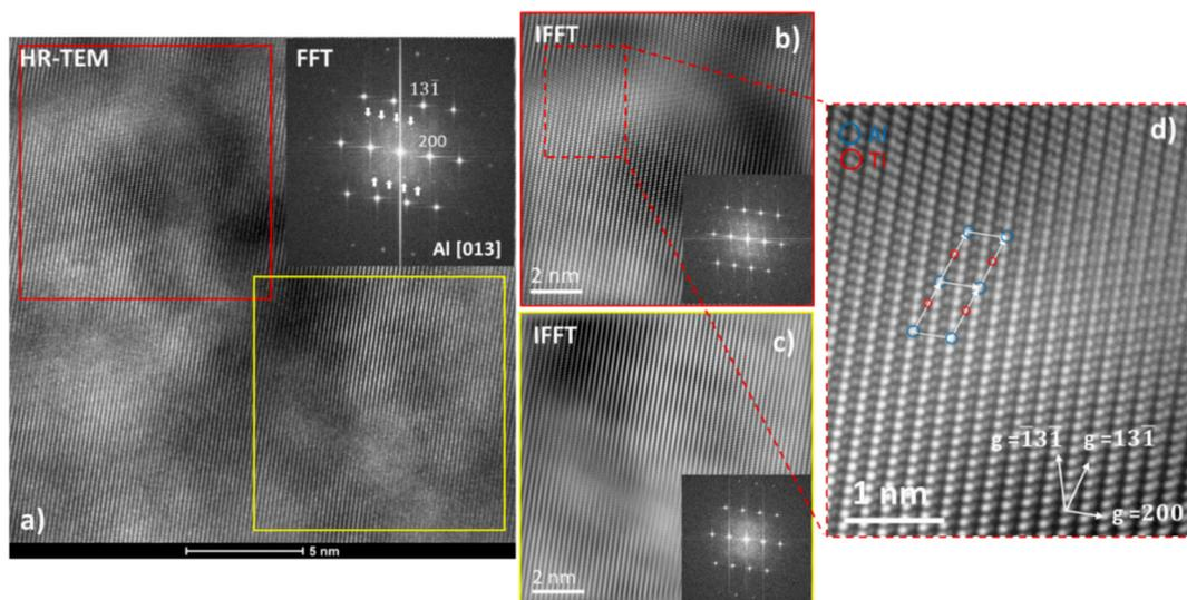
Fig. 9. (a) HR-TEM image and (b) corresponding reduced FFT, IFFT image generated from the red area in HR-TEM image, (c) IFFT image obtained from yellow area in HR-TEM image and (d) magnified area marked by red rectangle of IFF image. (For interpretation of the references to colour in this figure legend, the reader is referred to the web version of this article.)
