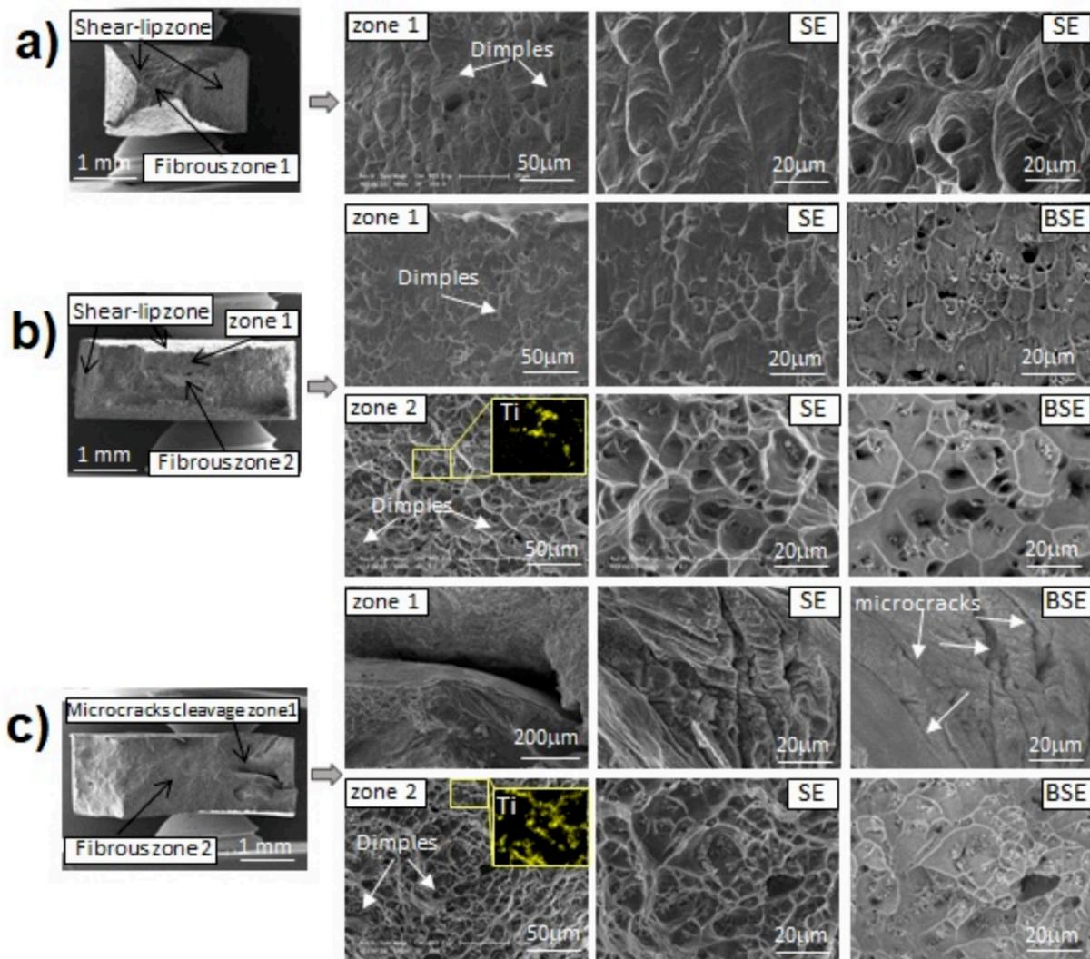
Fig. 13. Fracture surface of samples after tensile tests for a) the initial aluminum alloy, b) composite containing 5 vol% of TiC particles c) composite containing 15 vol% of TiC particles.
