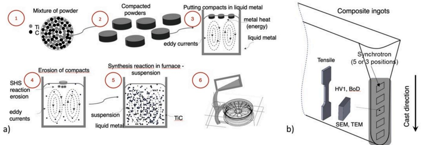
**Fig. 1.** (a) Casting concept showing the individual steps of the in situ process. (b) Sample cutting scheme indicating the locations from which the samples were spark-eroded.
