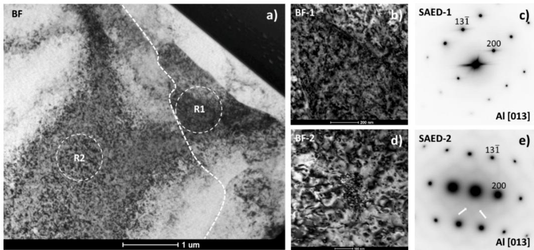
Fig. 7. (a) Lower magnification BF image and BF microstructures from regions R1 and R2 acquired with higher magnification (b), (d) and corresponding SEAD patterns (c), (e), respectively.
