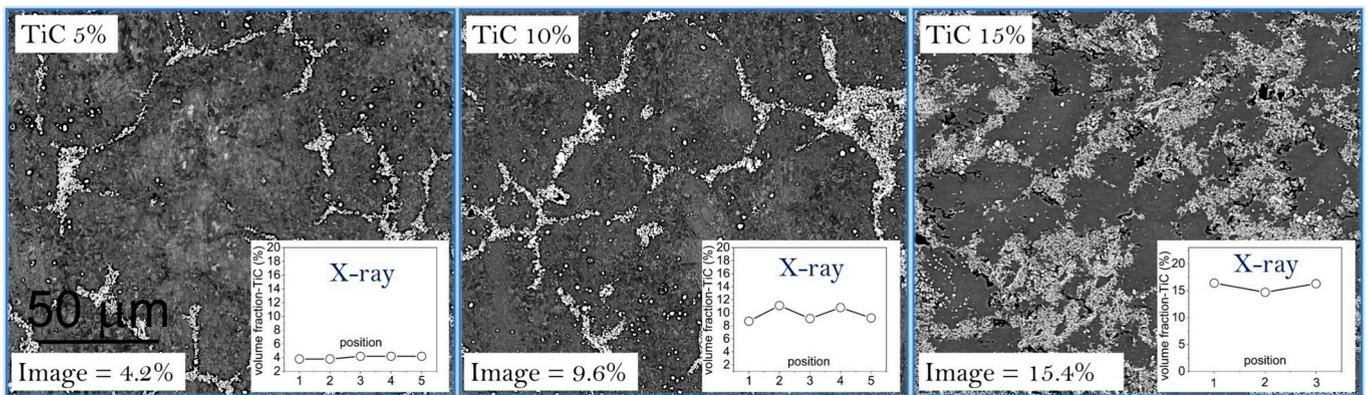
Fig. 4. Series of SEM-BSE images for samples with nominal TiC contents of 5%, 10%, and 15%, together with the corresponding TiC volume fractions calculated based on X-ray diffraction data and image analysis.
