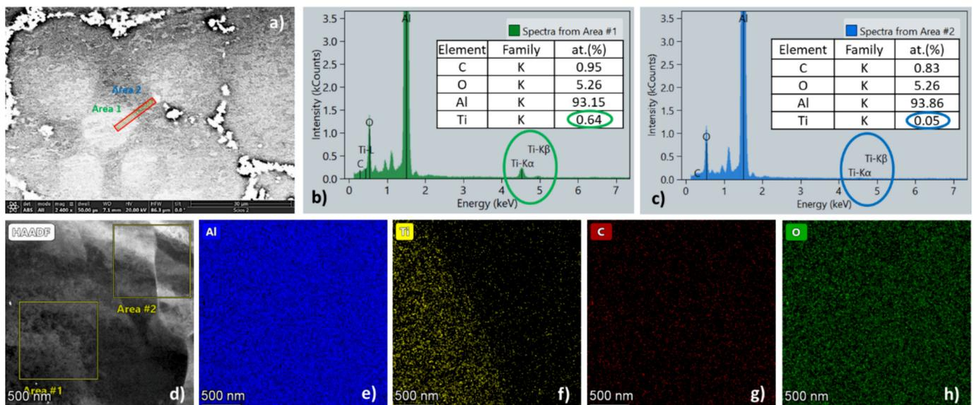
Fig. 6. (a) SEM BSE image with marked location of lamella cutting, (b) and (c) chemical composition results of taken from both Area 1 and Area 2, (d) STEM-HAADF image with marked both areas and (e-h) elemental mapping.
