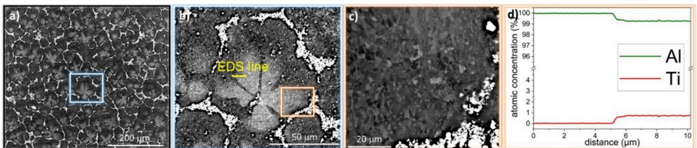
**Fig. 2.** (a–c) SEM images acquired in backscattered electron (BSE) mode of composite with a nominal 5 vol% of TiC at different magnifications, revealing characteristic compositional contrast variations within the dendritic grains; (d) EDS line scan performed along the yellow line marked in Fig. 1b. (For interpretation of the references to colour in this figure legend, the reader is referred to the web version of this article).
