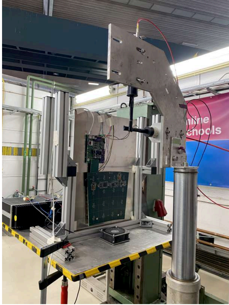
Figure 4.4: Picture of the movable stage and the trigger scintillators used during test beam campaigns. Courtesy of Jia-Hao Li.
