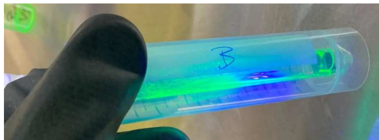
Figure S4. Photograph of the test tube after the two-layer phase diffusion assembly using acetonitrile antisolvent, showing NCs both adhered to the inner wall of the test tube and deposited on the Si substrate at the bottom of the test tube (right side of this rotated image). The residual acetonitrile phase was removed prior to the photograph.
