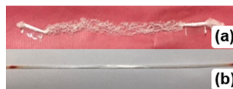
Fig. 2. (a) Unloaded and (b) weight-loaded (using fiber stretching frame setup) PLA fiber bundles of 150 single fibers after thermal treatment above T_g (80 °C).
