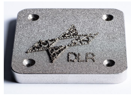
Fig. 1 View of the flight sample built during the MAPHEUS-10 sounding rocket flight. The thickness of the sample is limited to eight-layers due to the available microgravity time of 6.5 min. The build is completely welded to the platform without detaching. The sample thickness mildly decreases toward the right half, due to feed-stock particle transport coming in from the left
