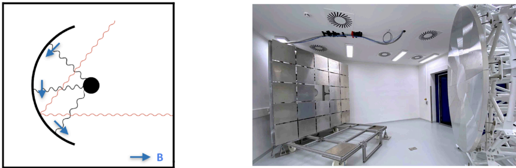
Figure 7: Dish antenna axion haloscope concept [54] (left) and picture of BRASS (right).
