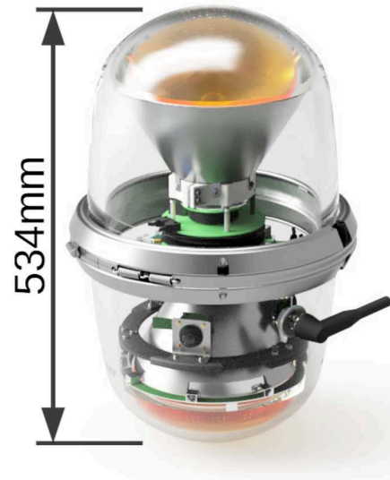
(b) CAD rendering of an assembled D-Egg. The annular PCB comprising the LED calibration system can be seen resting in the optical gel gluing the lower PMT to the glass pressure vessel.
