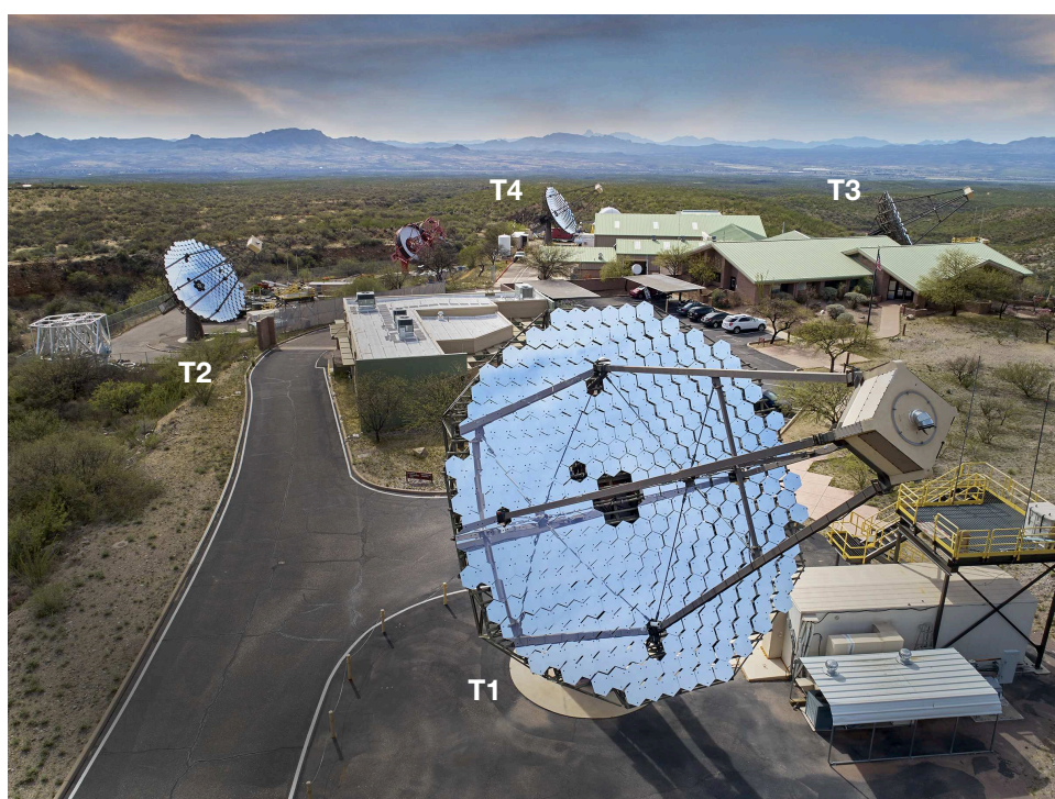
Figure 3.1: The Very Energetic Radiation Imaging Telescope Array System. The array consists of four telescopes, which are numbered in the image (T1, ..., T4). Credit: Center for Astrophysics - Harvard and Smithsonian (Adapted)
