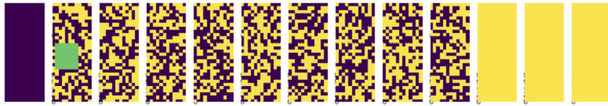
Fig. 4. Example: a passive volume in horizontal cross-sections starting from the bottom layer to the top. Yellow voxels indicate air, blue scrap metal, and green uranium. (For interpretation of the references to color in this figure legend, the reader is referred to the web version of this article.)
