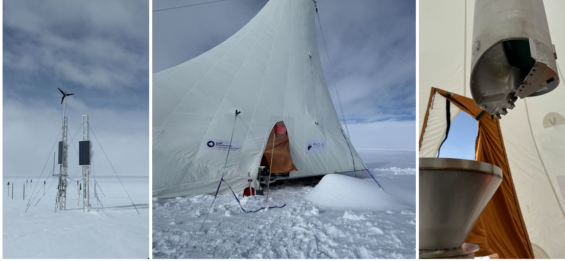
Figure 2: Impression of the RNO-G installation. Left: View of an installed station. From the outside, only the towers providing power and communications are visible. Middle: Drilling tent at the RNO-G site on June 10th 2025. The mount in front of the tent, stems from ice chips that are expelled from the drilling barrel. Right: View into the drilling barrel, showing one of the mechanical cutter-heads. With the limited infrastructure at Summit Station, the relatively shallow depths, and the large scales of the radio array, a hot-water drill is considered unfeasible.
