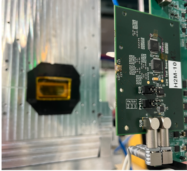
Figure 6.5: Photograph of H2M (right, foreground) and an ALPIDE telescope plane (left, background), illustrating the notable difference in sensitive area between the two sensors.
