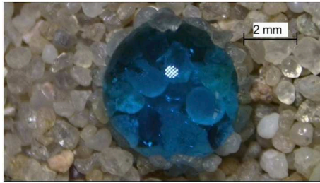
Fig. 1. Coloured water droplet resting on the surface of hydrophobic sand.
