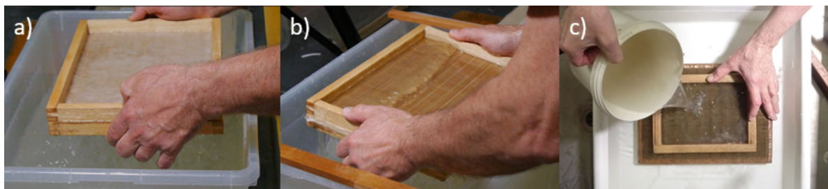
Fig. 3 Three historical sheet formation methods; Dipping method (left): Fibers are deposited onto the sieve by a single dip of the papermaking mold into the vat, which is then immediately lifted. Scooping method (center): Also known as nagashi-zuki , where fibers are
