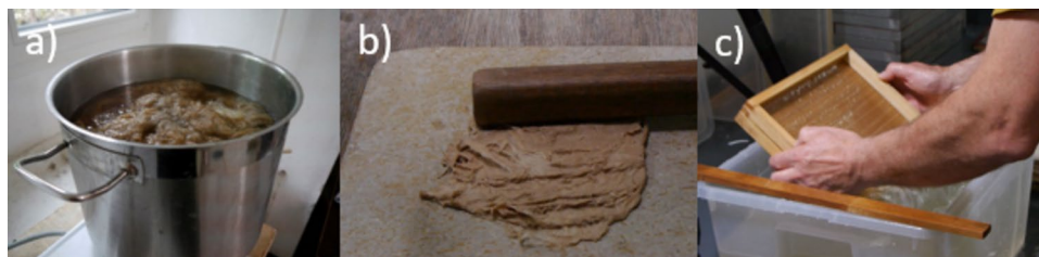
Fig. 1 Selected stages of the traditional papermaking process: Cooking plant fibers in an alkaline solution to remove non-cellulosic fractions and improve fiber bonding (a) manual beating of the fibers with a wooden mallet to further loosen the fibrillar fiber structure
