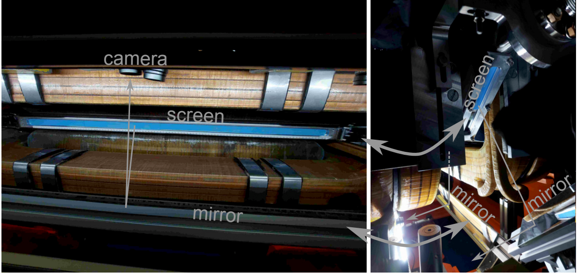
Figure 3.7: Left: picture of the 1-m-long low-energy screen, taken from below the dipole. A ruler for spatial calibration can be seen placed right below the screen. Right: picture of the high-energy screen, taken from the side, where the cameras are not visible. The double arrows show the same components in the pictures. In both cases, the signal emitted from the screen scintillator (blue) is reflected on a mirror to the cameras, as shown with the single gray arrows.
