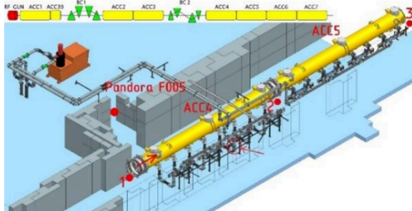
Figure 3: An overview of ACC4 and ACC5 cryomodules RF distribution. Red dots are X-ray sensors 1,2,3. The circle shows the position of the inserted attenuator for cavity 5 of ACC4.
