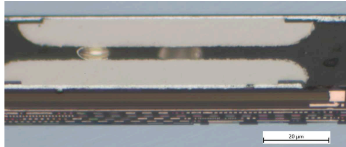
Figure 8. Microscopy picture of the cross-section for an ALTIROC2/LGAD device. The connection shown is from row 10 and pad number 7. It shows clearly two particles of 10 \mu\text{m} diameter being strongly squished between two ENIG coated pads.
