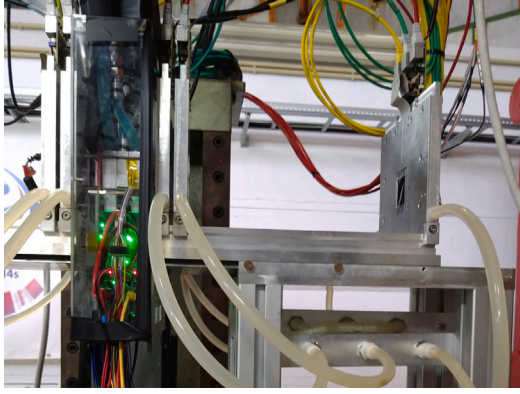
Fig. 8. Test-beam setup used in March 2023. The transparent plastic on the left contains the dSiPMs in their aluminum casing, the CaR board, and tubes for the light blue coolant. The five aluminum casings on the left and right contain the MIMOSA 26 sensors.
