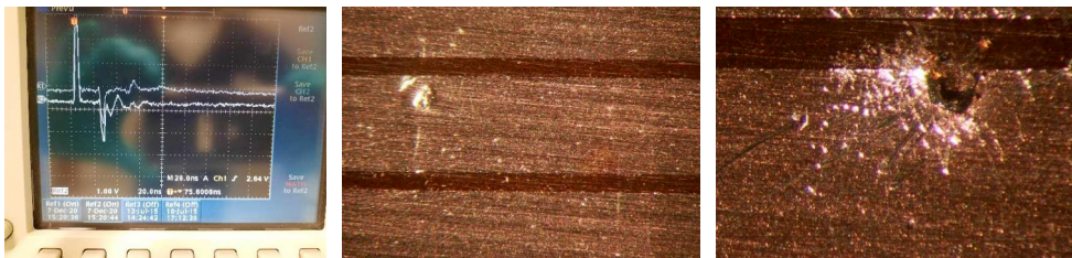
Fig. 6. a) TDR signals of a good and the faulty strip. b) Fault location. c) Opened hole (gap: 0.5 mm).
