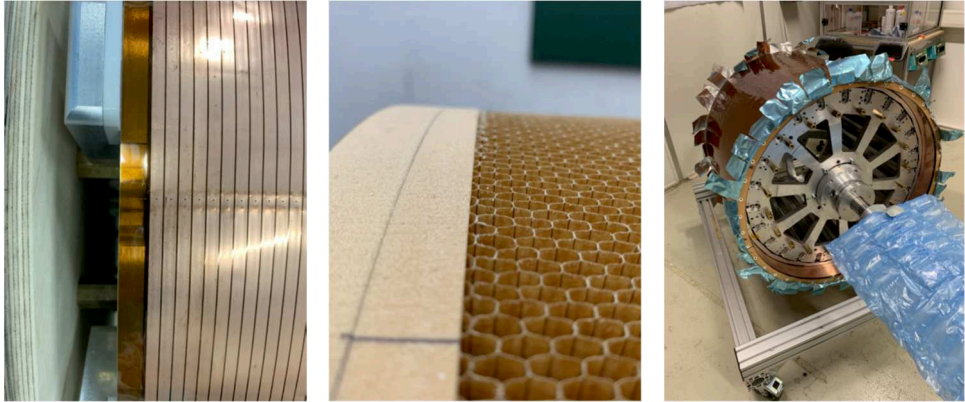
Fig. 11. a) Alignment of field strip foil. b) Routed flange honeycomb transition. c) Completed field cage being removed from the mandrel.
