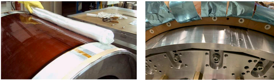
Fig. 2. a) Old mandrel during lamination. b) New mandrel in collapsed state.
