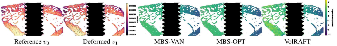
Figure 4. Evaluation of the measured volumes of PEEK_4w_5L, based on the reference volume (first) and the real deformed volume (second). Displacement fields are estimated by (from left to right): MBS-VAN [7] (third); MBS-OPT (fourth); the proposed VoIRAFT approach (fifth, the last one at the right). Cross sections (slices) of volumes and displacement fields are shown here.
