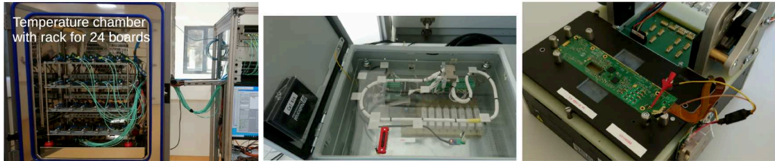
Figure 3. Test setups used for QC. Left: Climate chamber with rack of 24 EoS cards. Center: HV test setup. Right: Needle probe for electrical and optical connection tests.
