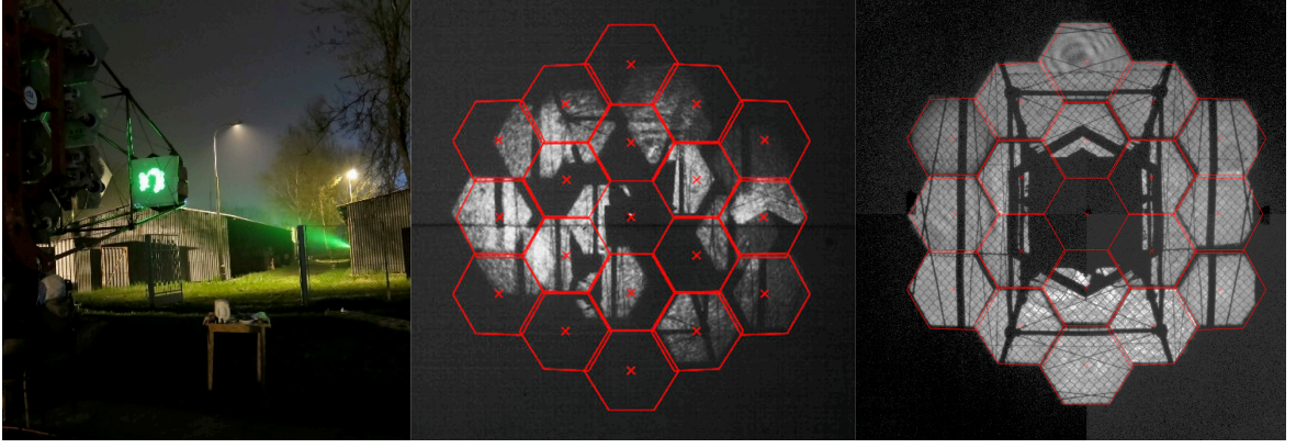
Figure 29. Setup for mirror alignment using the Bokeh method at the SST-1M prototype (left). The point-like laser source is placed at a distance of about 30 m, illuminating the screen placed in front of the telescope camera. The image of the close-distance point source is simulated and the individual mirror facet point source images are moved to a given position on the screen. The middle and right pictures show the facet images before and after alignment, respectively.
