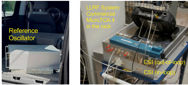
FIG. 11. Reference oscillator (left) was located outside the facility to reduce the influence of acoustic disturbances. The in-loop and out-of-loop CSI (right) are placed next to the rack, which houses the conventional LLRF system. On top of the modules, the baseband detection and a spectrum analyzer to track the quality of the carrier suppression are shown.
