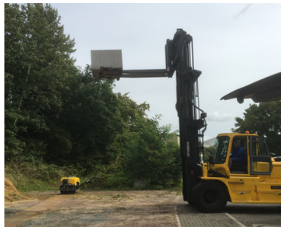
Figure 6: Dropping a 2-ton shielding stone from 5m height in the North area of the PETRA ring. The PETRA tunnel is only few ten meters away, below the rising ridge on the left side of the picture.
