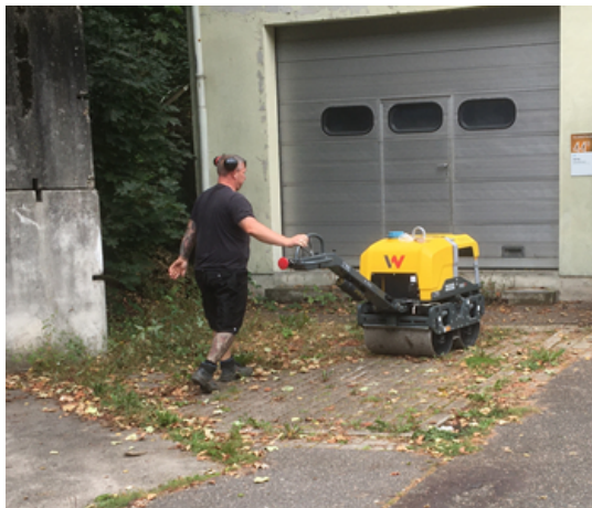
Figure 5: Ground excitation with a vibrating roller in the West area of the PETRA ring. The PETRA tunnel lays only a few meters to the left. The shielding stones in front of the material side entrance are visible on the left side of the picture.
