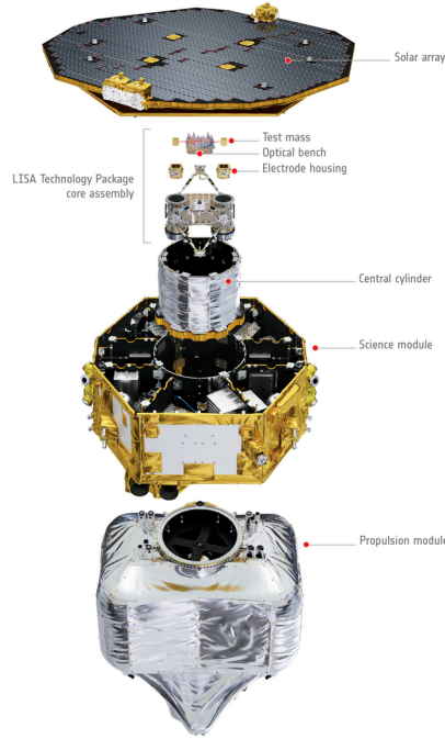
Figure 5.4: Exploded view of LPF showing the science module containing the test masses in its centre as well as the propulsion module. The technology package contains all of the experimental setup relevant to our analysis but since the entire mass of the SC goes into the calculation, we cannot completely ignore the structure or the solar panel. For simplicity, we will just perform a conservative estimate (see text). Image by ESA/ATG medialab (with permission).
