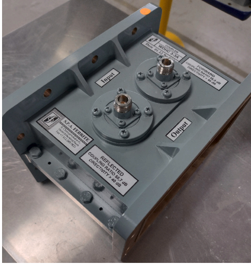
Fig. 1. S.P.A. FERRITE, WDHC 3-3A bi-directional coupler for 1.3 GHz waveguides. The declared directivity is 40 dB.
