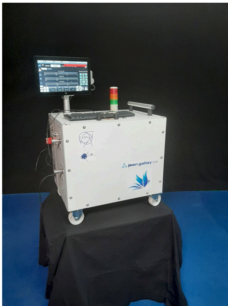
Figure 7. First of four prototypes to be produced in industry, to verify the HEV design parameters and optimize the form factor.
