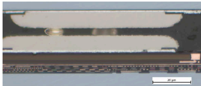
Figure 8. Microscopy picture of the cross-section for an ALTIROC2/LGAD device. The connection shown is from row 10 and pad number 7. It shows clearly two particles of 10 µm diameter being strongly squished between two ENIG coated pads.
