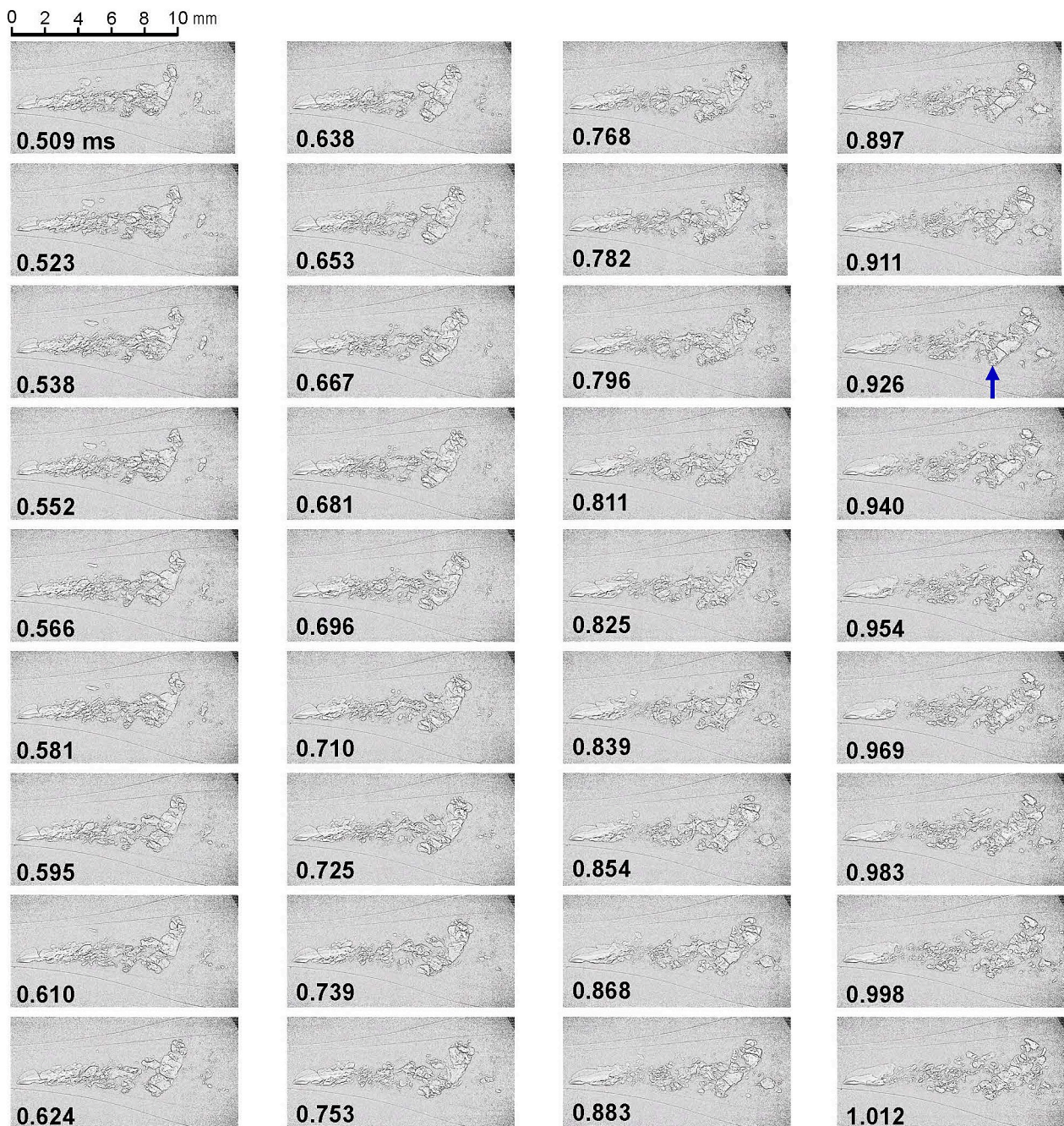
Fig. 10. One cycle of typical vortex cavitation from shedding of trailing edge to collapse at d = 2.0 mm, p_1 = 0.078 MPa, p_2 = 0.027 MPa, \sigma = 0.47 observed by high speed X-ray imaging.
