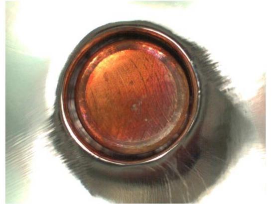
FIG. 6. Photograph of the inner surface of the back wall of a photoinjector cavity with inserted copper cathode plug.
