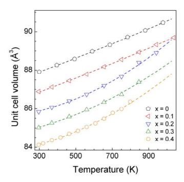
Fig. 7 Unit cell volumes of rs-Mn<sub>1-x</sub>Zn<sub>x</sub>O solid solutions versus temperature at ambient pressure. Error bars are smaller than the symbols. Dashed lines are least squares fits (see Table 3).
