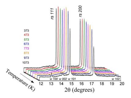
Fig. 1 Sequence of synchrotron powder X-ray diffraction patterns ( $\lambda$  = 0.6515 Å) of Ni<sub>0.2</sub>Zn<sub>0.8</sub>O solid solution taken during stepwise heating to 1100 K. The rock-salt phase is stable up to ~970 K; the decomposition products are a mixture of two solid solutions, wurtzite and cubic.
