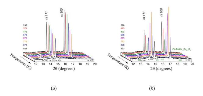
Fig. 3 Sequence of synchrotron powder X-ray diffraction patterns ( $\lambda = 0.6515 \text{ Å}$ ) of rock-salt  $Co_{0.3}Zn_{0.7}O$  (a) and  $Co_{0.4}Zn_{0.6}O$  (b) solid solutions taken during stepwise heating to 950 K. The first solid solution converts completely to a wurtzite structure, while the decomposition products of the second are a mixture of three phases - wurtzite, cubic and spinel-like.
