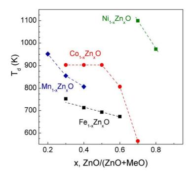
Fig. 10 Comparison of phase stability of rock-salt ZnO-MeO (Me = Ni, Co, Mn, Fe) solid solutions at ambient pressure. Below the dashed lines are the fields of kinetic stability of the corresponding cubic phases; above them the decomposition with formation of different phases is observed.
