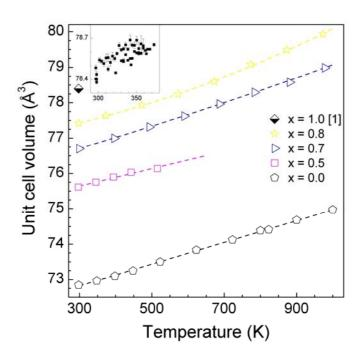
Fig. 2 Unit cell volumes of *rs*-Ni<sub>1-x</sub>Zn<sub>x</sub>O solid solutions *versus* temperature at ambient pressure. Error bars are smaller than the symbols. Dashed lines are least squares fits (see Table 1). Inset: small symbols correspond to our data on lattice parameters of nanocrystalline rock-salt ZnO in the 300-370 K range.
