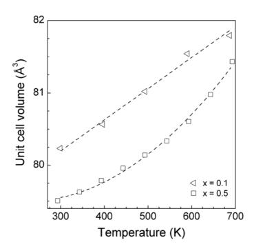
Fig. 9 Unit cell volumes of rs-Fe<sub>1-x</sub>Zn<sub>x</sub>O solid solutions versus temperature at ambient pressure. Error bars are smaller than the symbols. Dashed lines are just guides for the eye.
