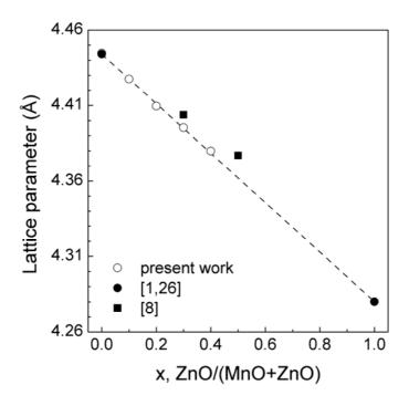
Fig. 5 Lattice parameters of rs-Mn<sub>1-x</sub>Zn<sub>x</sub>O solid solutions as a function of composition.
