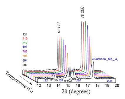
Fig. 6 Sequence of synchrotron powder X-ray diffraction patterns ( $\lambda$  = 0.6882 Å) of Mn<sub>0.6</sub>Zn<sub>0.4</sub>O solid solution taken during stepwise heating to 1000 K. The initial rock-salt phase is stable up to 850 K; the decomposition products are a mixture of three phases - wurtzite, cubic and spinel-like.
