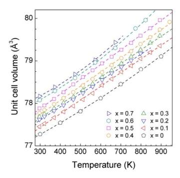
Fig. 4 Unit cell volumes of rs-Co<sub>1-x</sub>Zn<sub>x</sub>O solid solutions versus temperature at ambient pressure. Error bars are smaller than the symbols. Dashed lines are least squares fits (see Table 2).
