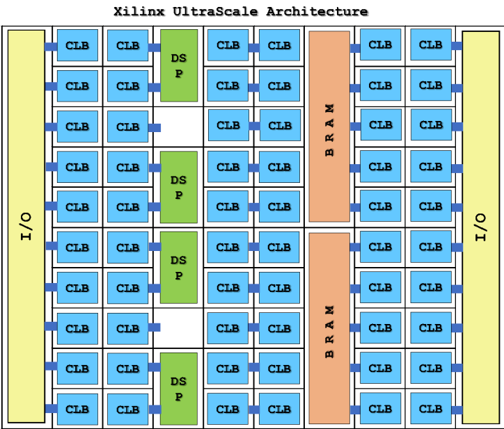
Figure 9. The architecture of the Xilinx UltraScale FPGA accelerator card.
