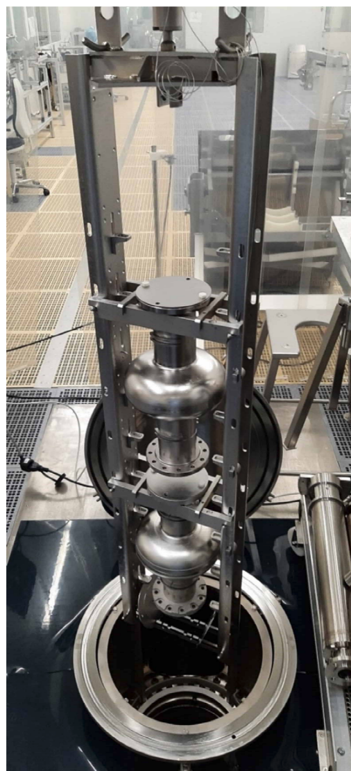
Figure 6: Furnace frame equipped with two single-cell cavities.
