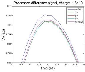
Figure 8: FONT BPM processor output near the signal peak for beam runs without, and with, thin radiators in place. Each curve is the average over 1000 beam pulses.
