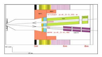
Figure 1: Schematic of ILC interaction region showing possible locations of the kicker and BPM.
