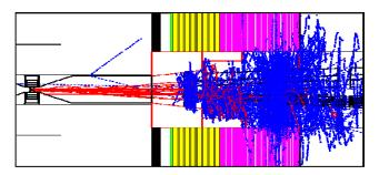
Figure 2: Example of primary e+e- pair particles striking forward-region elements and causing secondary EM showers in the vicinity of the IP feedback BPM.
