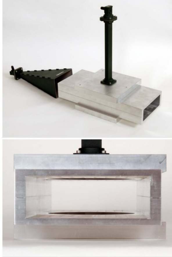
Figure 5: Nearly confocal resonator prototype inserted onto a rectangular Aluminium pipe, with its extraction waveguide. The horn antenna used to inject external modes into the nearly confocal resonator through the pipe is shown in the upper picture. Also, one can clearly see the two carved spherical mirrors in the lower picture.
